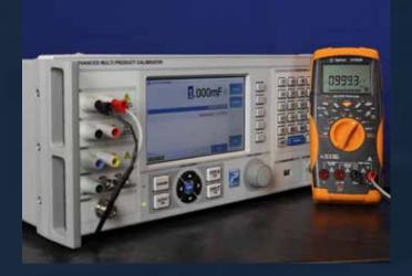
Included in -SYS units, the simulated option provides for resistance calibration between cardinal points and gives a continuous resistance range from 0 Ohms to 1 GOhms, with variable capacitance from 0.95uF through to 100mF.
