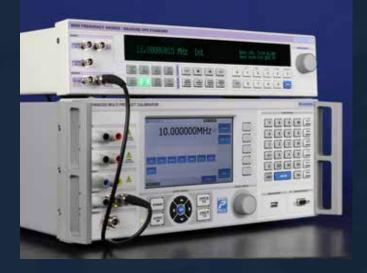
For calibration of high accuracy frequency counters, a 1ppm high stability frequency output is available (Included in 4010)
